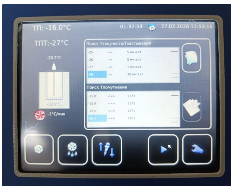
Fig. 4. Low-temperature fuel properties were determined using the TPZ-LAB-12
